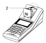
Pull up the height adapter (3). The cell shaft is extended.
